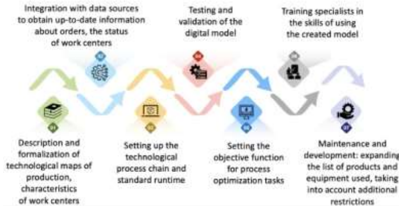
Figure 8. The stages of digital twin construction
